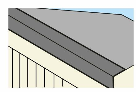
Step Three – Eaves and Verge Detailing. Cut strips from the shingles pieces and fix to roof using galvanised clout nails so that the strips overhang the gable and eaves edges by 50mm
