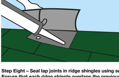
Step Eight – Seal lap joints in ridge shingles using suitable mastic or felt adhesive. Ensure that each ridge shingle overlaps the previous one, exposing approximately 145mm. Continue to fix the ridge shingles along the roof ridge using galvanised clout nails, bending lengthways down the centre of the roof to achieve equal exposure on both sides of the ridge. Warm the shingles before folding in cold weather to avoid cracking the membrane.
