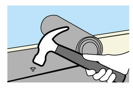
Step Two – Fix a 1m wide universal underlay across the width of the roof and fix at 500mm centres using galvanised clout nails
