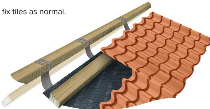
**NOTE:** If at this stage it is acknowledged that the brackets were not set high enough at stage 1, then another batten can be screw fixed on top of the original to achieve correct engagement.
