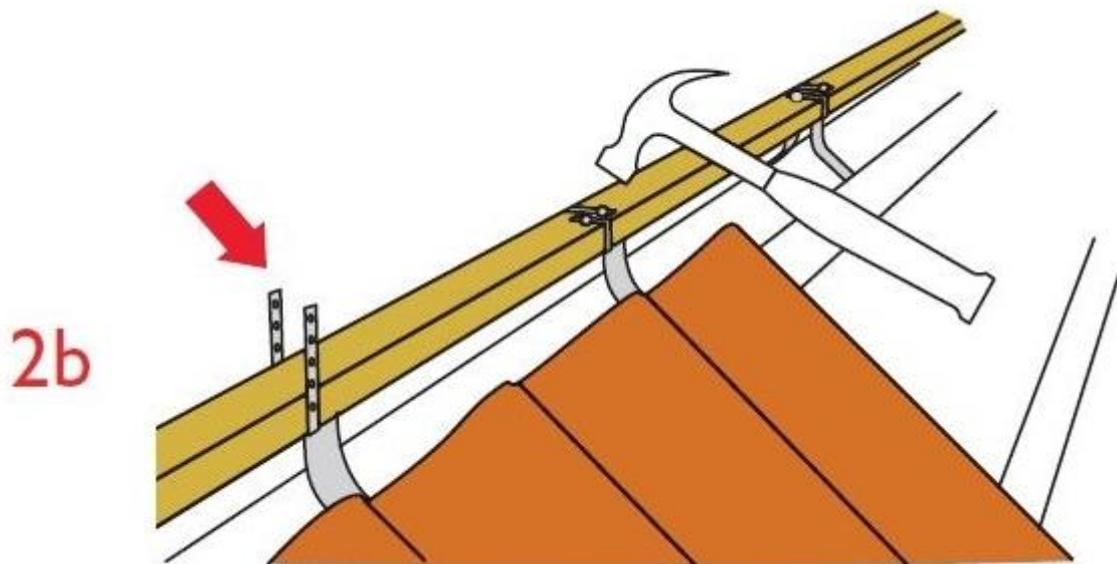
**3.** Unroll ridge-roll and fix with a nail at 1-2m centres. *Ridge roll should overlap at edge of gable end by approx. 50mm when using a dry verge or block end ridge tile. When using a bedded verge, stop ridge roll 50mm short from edge of gable end.*
