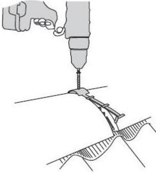
NOTE: If at this point it is discovered that the brackets were not set high enough at stage 1, another batten can be screw fixed on top of the original to achieve correct engagement. Ensure additional batten does not block vent holes in ridge roll.
